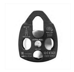
Aluminum pulley with single wheel, mobile side plates and high efficiency (96%) ball bearing. Equipped with two attachment points for use in complex lifting systems.
