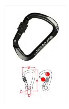
Light alloy carabiner with screw sleeve. The X-Large is designed to offer a wide gate opening and a high tensile strength. The particular D shape prevents the rotation of the carabiner and allows to distribute the load along the major axis.
