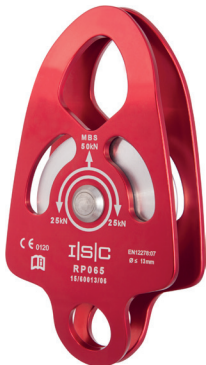
RPo65 Medium Single Prussik Weight 215g (8oz) Max. Rope Diameter 13mm (1/2") MBS 50kN (11240lbf) Becket Yes
