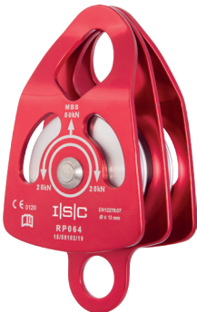
RPo64 Medium Double Prussik Weight 500g (17.6oz) Max. Rope Diameter 13mm (1/2") MBS 50kN (11240lbf) Becket Yes
