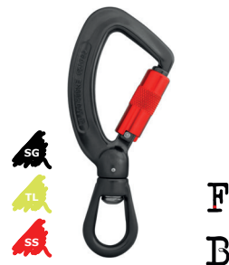
KH255 Twister Weight 142g (5oz) Gate Opening 15mm (5/8") MBS 27kN (6070lbf) Height 175mm (6 7/8") Width 72mm (2 7/8")
