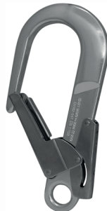
SH979 Large Scaffold Snaphook Weight 514g (18oz) Gate Opening 65mm (2 1/4") MBS 25kN (6070lbf) Gate Type Double Action Material Aluminium
