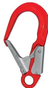
SH999 Large Scaffold Snaphook Weight 495g (17oz) Gate Opening 65mm (2 3/8") MBS 35kN (7868lbf) Gate Type Double Action Material Aluminium
