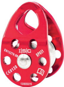
RP031 Double Re-direct Pulley Weight 124g (4oz) Max. Rope Diameter 13mm (1/2") MBS 30kN (6744lbf) Wheel Material Aluminium
