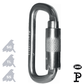
KH308 D Shape Weight 174g (6oz) Gate Opening 16mm (5/8") MBS 22kN (4946lbf)
