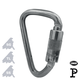
KH202 Klettersteig Weight 269g (9.5oz) Gate Opening 22mm (7/8") MBS 35kN (7868lbf)
