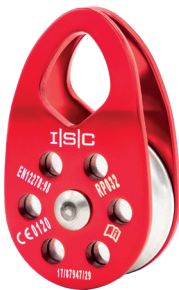
RP032 Medium Single Pulley Weight 158g (6oz) Max. Rope Diameter 13mm (1/2") MBS 36kN (8093lbf) Wheel Material Aluminium
