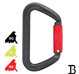
KH218 Aluminium Wizard Weight 113g (4oz) Gate Opening 29mm (1 1/8") MBS 40kN (8992lbf) Height 128mm (5") Width 73mm (2 7/8")
