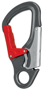
SH901 Standard Snaphook Weight 130g (4.6oz) Gate Opening 23mm (7/8") MBS 27kN (6070lbf) Gate Type Double Action Material Aluminium
