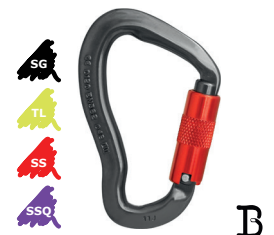
KH452 Gecko Weight 86g (3oz) Gate Opening 21mm (7/8") MBS 30kN (6744lbf) Height 115mm (4 1/2") Width 75mm (3")
