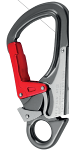
SH903 Standard Snaphook Weight 135g (4.8oz) Gate Opening 23mm (7/8") MBS 27kN (6070lbf) Gate Type Triple Action Material Aluminium
