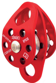
RP030 Small Double Pulley Weight 150g (5oz) Max. Rope Diameter 13mm (1/2") MBS 35kN (7868lbf) Wheel Material Aluminium
