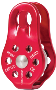
RP037 Micro Pulley Weight 90g (3oz) Max. Rope Diameter 13mm (1/2") MBS 28kN (6294lbf)
