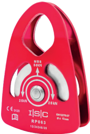
RP063 Medium Single Prussik Weight 215g (7.6oz) Max. Rope Diameter 13mm (1/2") MBS 50kN (11240lbf)
