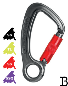
KH300 Captive Eye Weight 99g (3.5oz) Gate Opening 20mm (3/4") MBS 30kN (6744lbf) Height 137mm (5 3/8") Width 75mm (3")
