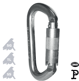
KH200 Offset D Weight 255g (9oz) Gate Opening 20mm (3/4") MBS 35kN (7868lbf)
