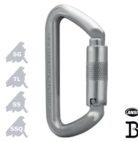
KH219 Wizard Weight 286g (10oz) Gate Opening 28mm (1 1/8") MBS 50kN (11240lbf)
