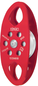
RP034 Medium Double Ended Pulley Weight 180g (6oz) Max. Rope Diameter 13mm (1/2") MBS 36kN (8093lbf) Wheel Material Aluminium
