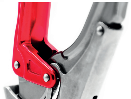
SH999 Large Scaffold Snaphook Weight 495g (17oz) Gate Opening 65mm (2 3/8") MBS 35kN (7868lbf) Gate Type Double Action Material Aluminium
