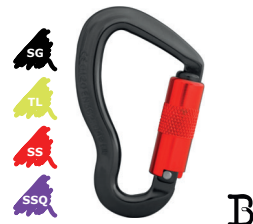
KH453 Gator Weight 47g (1.7oz) Gate Opening 15mm (5/8") MBS 25kN (5620lbf) Height 105mm (4 1/8") Width 65mm (2 1/2")
