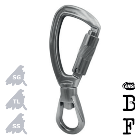
KH250 Twister Weight 374g (13oz) Gate Opening 18mm (3/4") MBS 23kN (5171lbf)
