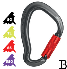
KH451 Mongoose Weight 118g (4.1oz) Gate Opening 24mm (1") MBS 30kN (6744lbf) Height 133mm (5 1/4") Width 88mm (3 1/2")
