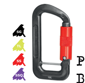
KH215 Link Weight 85g (3oz) Gate Opening 15mm (5/8") MBS 25kN (5620lbf) Height 113mm (4 1/2") Width 61mm (2 3/8")
