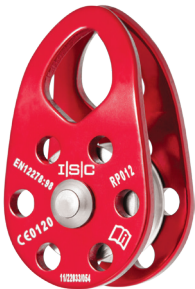
RP012 Small Single Pulley Weight 87g (3oz) Max. Rope Diameter 13mm (1/2") MBS 36kN (8093lbf) Wheel Material Aluminium
