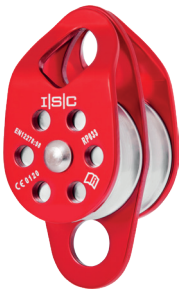
RP033 Medium Double Pulley Weight 284g (10oz) Max. Rope Diameter 13mm (1/2") MBS 36kN (8093lbf) Wheel Material Aluminium
