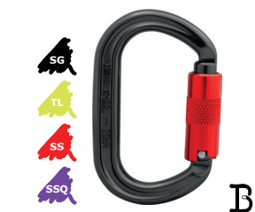
KH221 Oval Weight 86g (3oz) Gate Opening 19mm (3/4") MBS 25kN (5620lbf) Height 111mm (4 3/8") Width 67mm (3")
