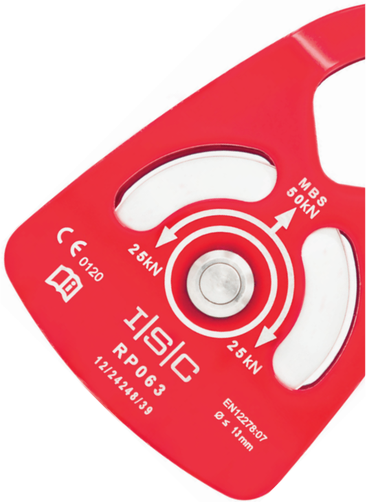
RP063 Medium Single Prussik Weight 215g (7.6oz) Max. Rope Diameter 13mm (1/2") MBS 50kN (11240lbf)
