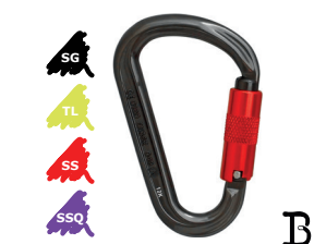
KH204 HMS Weight 103g (3.6oz) Gate Opening 19mm (3/4") MBS 27kN (6070lbf) Height 124mm (4 7/8") Width 78mm (3 1/3")
